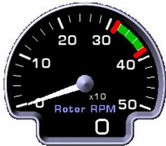
Indicator of ROTOR RPM
