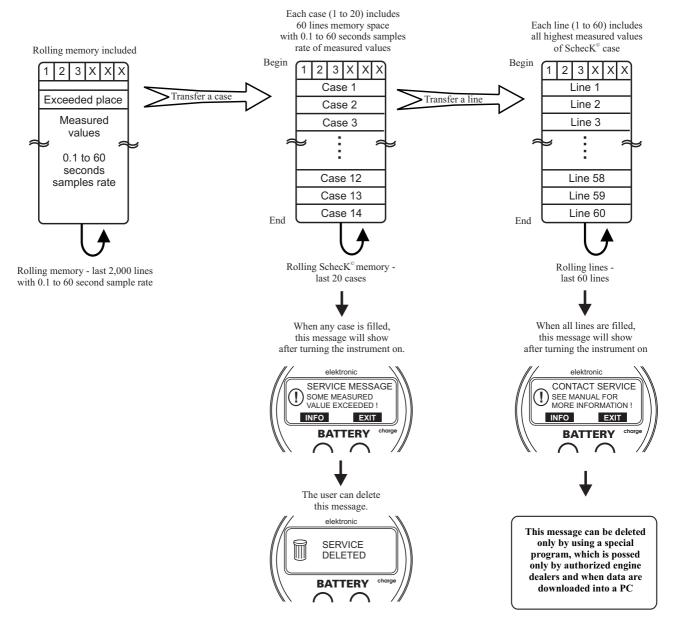
Cases 1 to 20 include 60 lines of exceeded limit values and engine hours when the values have been exceeded.
