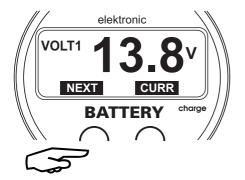
To store a value into the memory, press both buttons simultaneously. Release the buttons when the setting arrows vanish.
