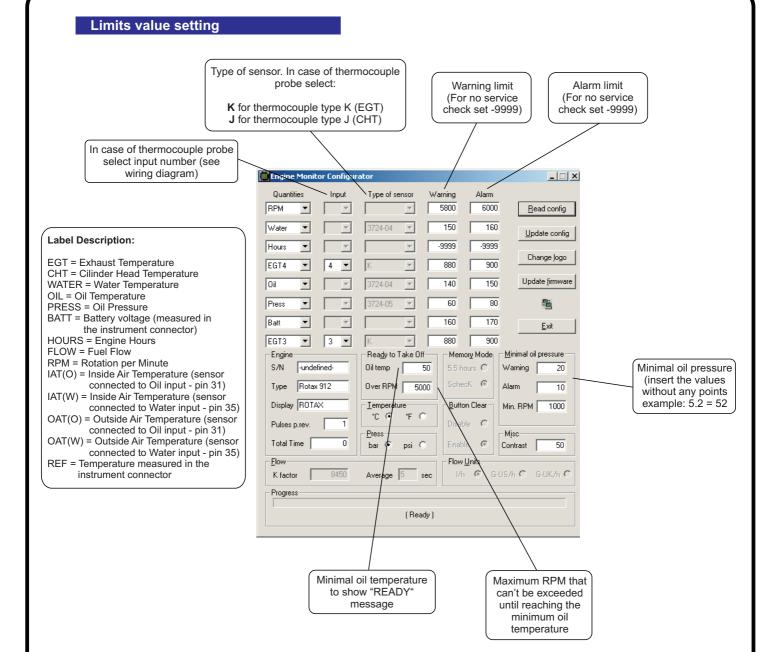
NOTE: Limit values of oil pressure, fuel pressure and battery voltage are written without any points. Always write the number in the form of ones and tenths.
